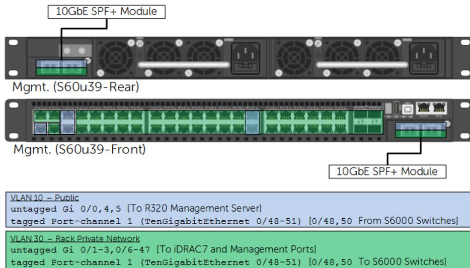
Figure 11 VLAN Configuration on the S60 Management Switch
