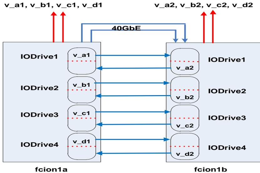
Figure 14 Storage volume setup on the DAAD Storage Array
