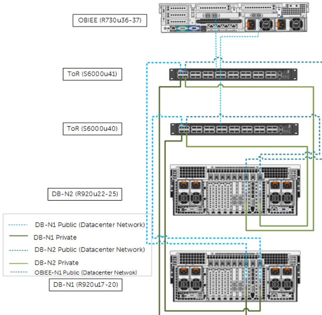
Figure 15 Cabling Diagram – LAN Infrastructure
