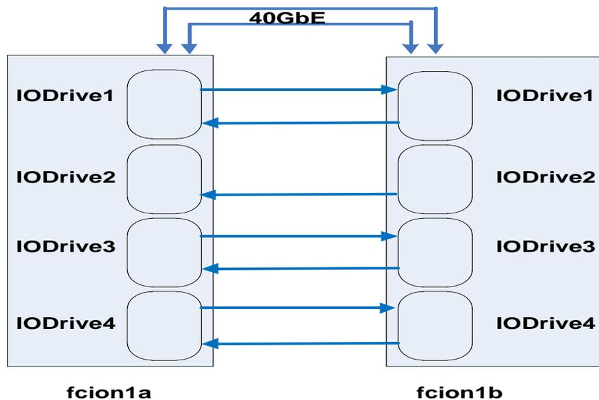
Figure 13 Mirroring between the ioMemory cards between the DAAD Storage Array nodes
