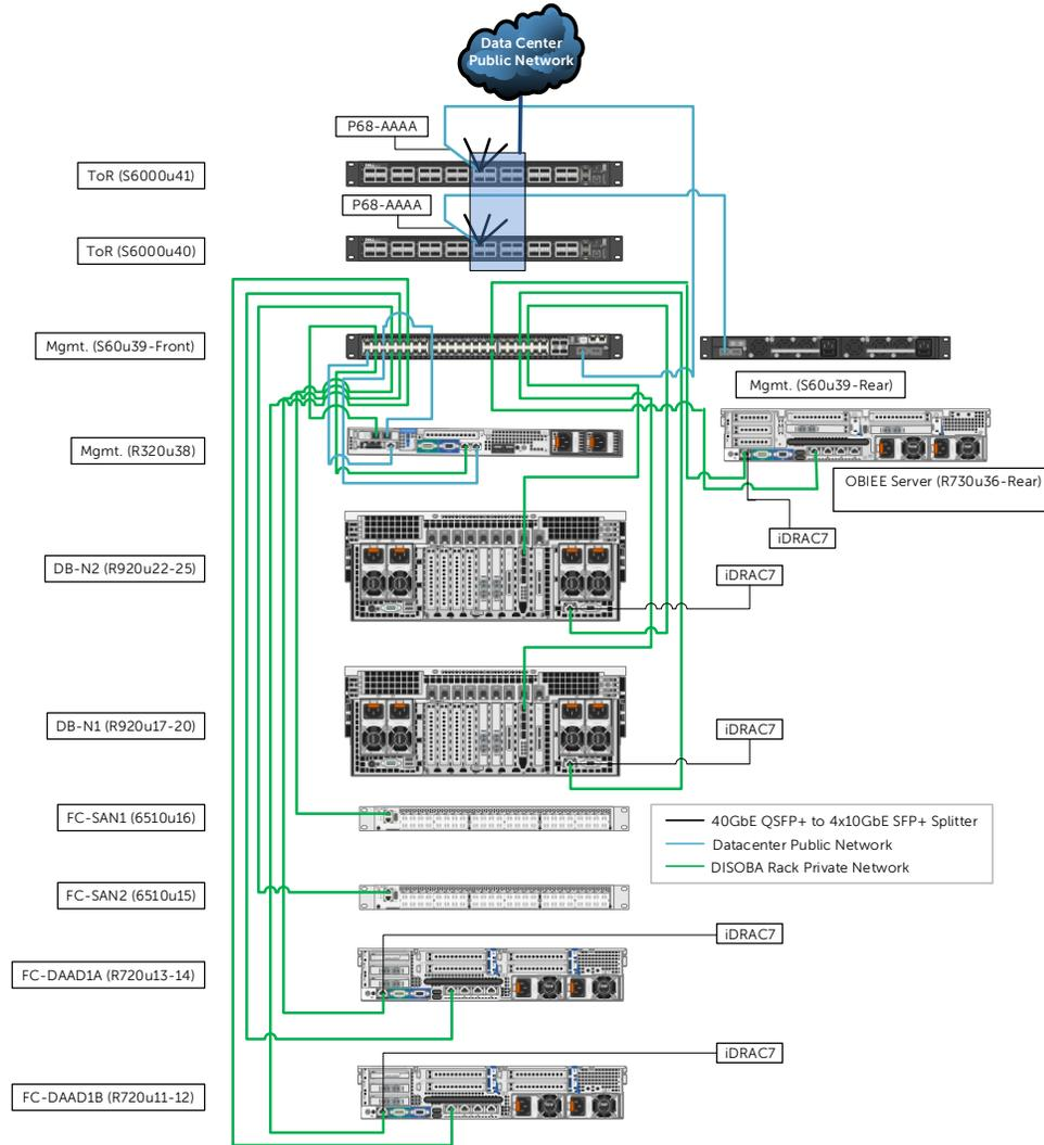
Figure 17 Cabling Diagram – Management Infrastructure
