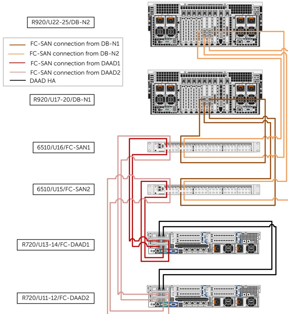
Figure 16 Cabling Diagram – SAN Infrastructure
