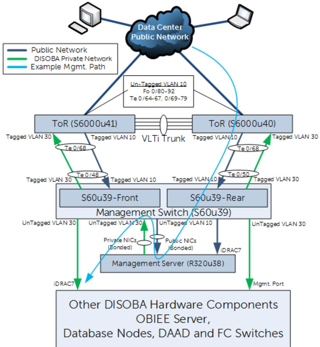
Figure 12 DISOBA Management and Monitoring Network
