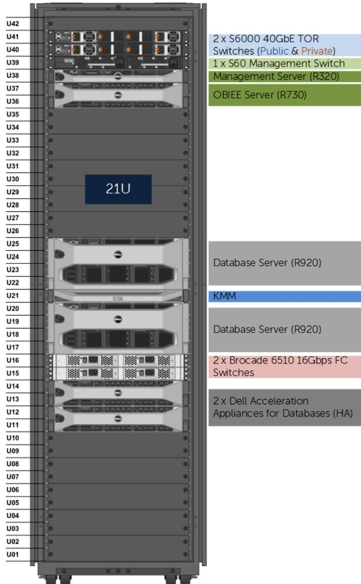
Figure 1 Dell Integrated Systems for Oracle Business Analytics (DISOBA) Hardware Rack
