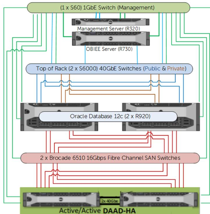
Figure 2 Architectural Diagram of DISOBA
