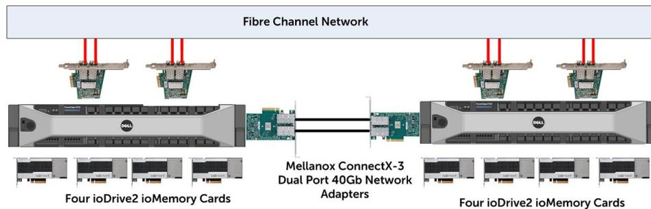
Figure 5 DISOD Shared Storage: Highly Available FC based DAAD Storage Array
