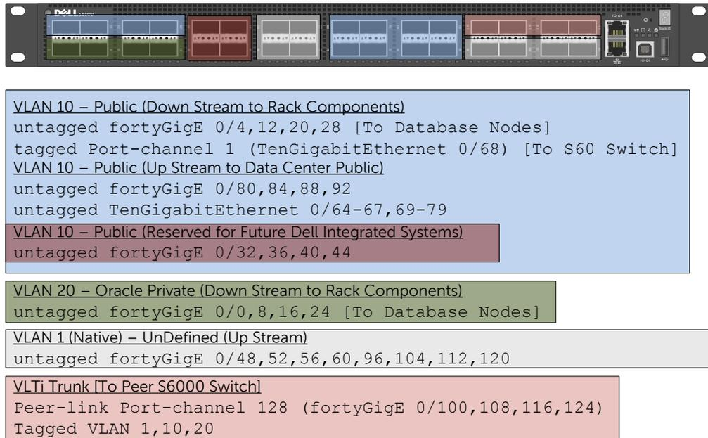
Figure 9 S6000 VLAN and Port Channel Configuration
