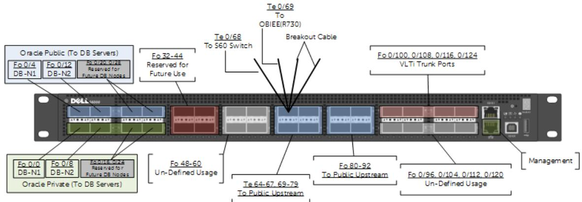
Figure 8 S6000 Port Functions and Configurations
