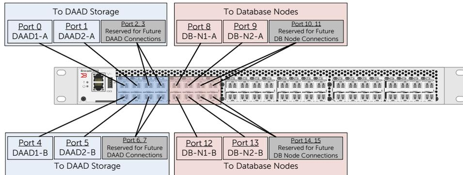
Figure 6 Brocade 6510 Fibre Channel Switch Port Connectivity
